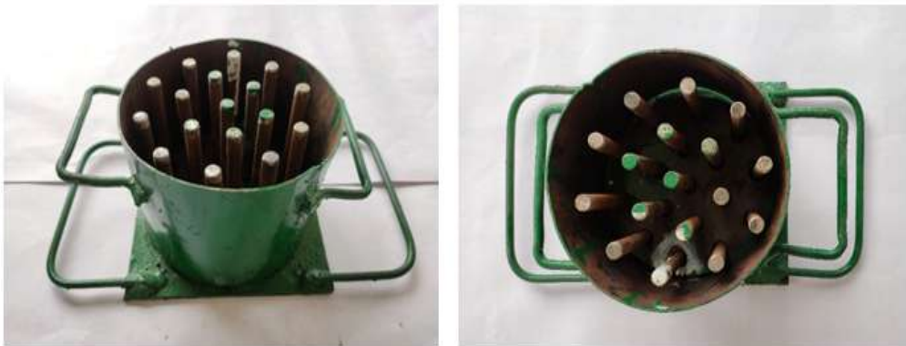
Fig. 1. Iron mould for making bio-briquettes
